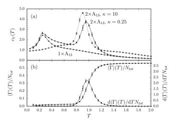
Fig. 1: (a) Specific heat per monomer as a function of temperature for a single semiflexible homopolymer with 13 monomers  $(1 \times A_{13}, \kappa = 0.25)$  and for systems of two such chains  $(2 \times A_{13})$  with different bending rigidities. (b) Canonical expectation value  $\langle \Gamma \rangle$  and fluctuation  $d\langle \Gamma \rangle/dT$  of the aggregation parameter  $\Gamma$ , defined in eq. (6), for the two-chain system with  $\kappa = 0.25$ .
